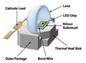
Red LEDs are based on aluminum gallium arsenide(AlGaAs).Blue LEDs are made fromindium gallium nitride(InGaN). Green LEDs from aluminum galliumphosphide (AlGaP). "White" light is created bycombining the light from red, green, and blue (RGB) LEDs. White - by coating a blueLED with yellow phosphor. Besides, an LED has:
