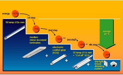
Fig. Energy saving by deploying dimmers
